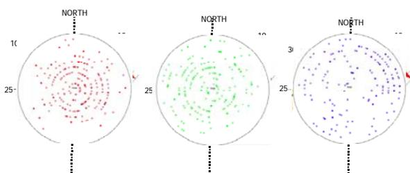
An example of the work undertaken by one of our associates is provide by Jon Heuch, of Duramen Consulting. Jon uses radar ground imaging techniques to detect roots above a certain diameter, and using software he is able to plot them by depth.
