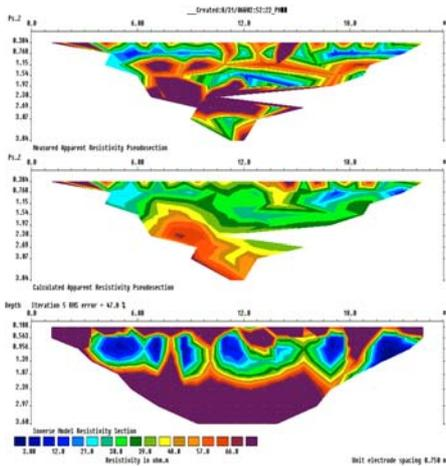
Measuring the resistivity of a soil provides an indication of its moisture content, and although this is a well researched topic, work on fine grained London clay is relatively new and very relevant to our understanding of how moisture moves in relation to root extraction.
