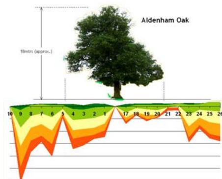
Precise levels have provided some invaluable information. Whilst other techniques measure specific elements, precise levels are the most efficient way of determining the combined interaction and effect of moisture change, root activity (including hormonal influence) and climate.
