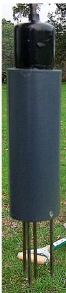
TDR sensors have been validated using comparisons with the neutron probe and ground movement and we are satisfied they provide a sensible record of volumetric moisture content.
