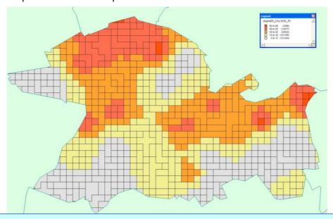
The CRG geology map plots the PI on a 250m grid and has been built from actual investigations. The soil PI is higher to the north of the Borough, with low shrinkability soils interspersed. The index properties have been taken from a depth of around 2mtrs wherever possible to coincide with the depth of maximum root activity for mature, deciduous trees.
