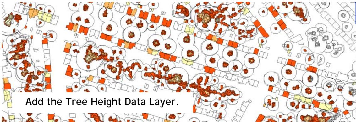
These images plot a sample from Sidcup Road with many trees planted around the same time. The risk rating is determined by matching colour coded houses with shaded trees nearby, the modelled root zones of which ‘touch’ the building, but do not cover the building footprint.
