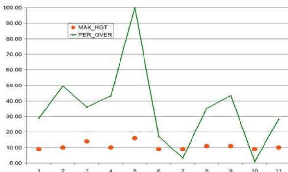
What can we see from the data? Is there a particular combination that presents a greater risk? How do damaged houses compare with undamaged houses? Of the 11 claims notified, 9 have trees of a height of around 10mtrs and 10 have root zones less than 50%. Only 1 has a root zone of 100%.
