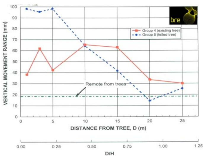
Interestingly, for both sets of rods, the greatest movements do not appear to occur at the point nearest the tree, but a few metres away. This is particularly noticeable for the rods emanating from the existing tree, where maximum magnitude of movement has occurred some 10m away from the tree.
