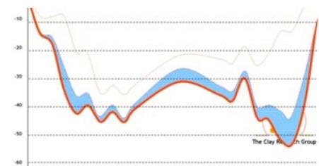
The trees are similar in height to the Aldenham Oak, the ground movement profile from which is shown above, revealing amplified movement at the root periphery.
