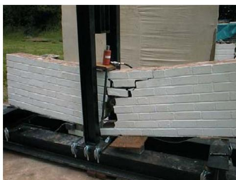
We already have parameters of masonry reinforcement and limiting tensile stresses from the work of Burland, Wroth, Skempton and others, plus the more recent research at the premises of C.P. Bennett in Solihull where masonry panels have been tested to destruction (left).
