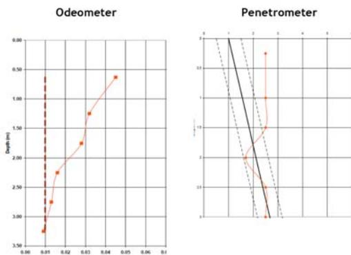
Desiccation down to 2mtrs, detected by both the oedometer (left) and penetrometer (right).
