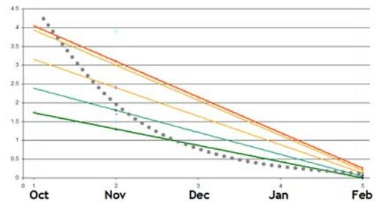
By adding ground movement profiles over time using the level data from the site of the Aldenham Willow we see how much movement takes place over time, and from this tree, on this site at this time, plotting month by month movement with the lowest profile recording the September profile.
