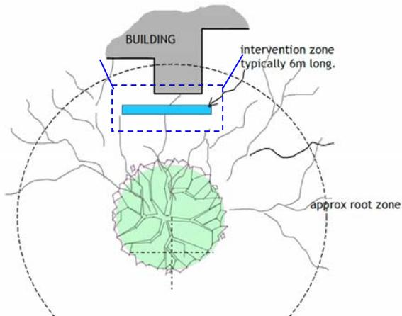
Reflecting on our aims, the treatment zone is almost certainly too small in relation to the root footprint of a mature tree to trigger production of the hormone, Abscisic Acid as part of the Partial Root Drying treatment, which means any benefit is related to local rehydration.
