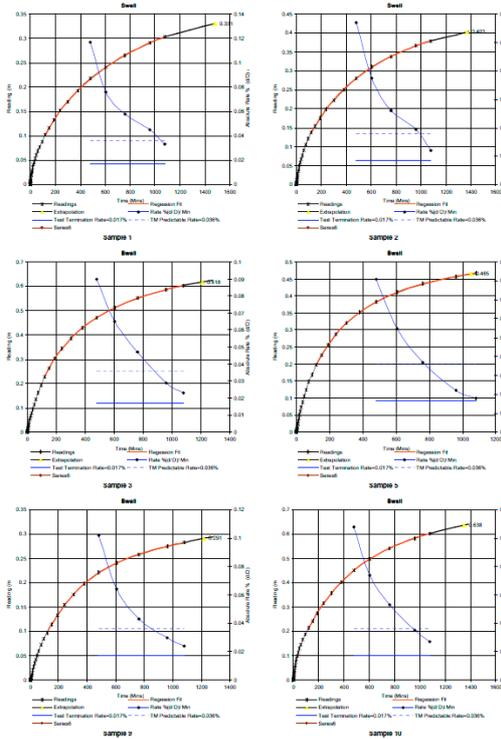
Predictive swell rates have been developed to safely shorten the test cycle when using the oedometer, as we see above.
