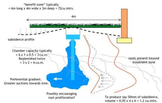
Dr Allan Tew suggests the deficit can be catered for by harvesting roof water rainfall of say 700mm over half the roof area of a typical house ( $20^2\text{m}$ , collected by guttering and diverted to the trench via a drainage system with auto-cut off, overflow facility and ventilation) delivers around  $14^3\text{mtrs}$ . Adjoining suctions will equilibrate the available moisture over a larger volume.
