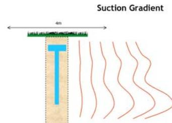
Increasing the notional zone to say 4mtrs, and assuming the treatment has to satisfy ground subsidence of 50mm for a short duration – a few months – the situation might be as shown below, with the chamber delivering 6 cu.mtrs of water to replace local loss over the treatment zone of 1.2 cu.mtrs.
