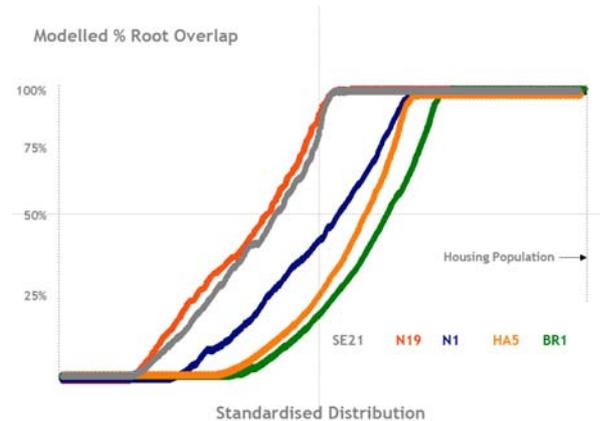
The above graph shows the modelled root overlap beneath buildings for a series of Boroughs. If we look at the red line for example (N19), we can see that around 13% of the houses have no estimated root encroachment at all.
