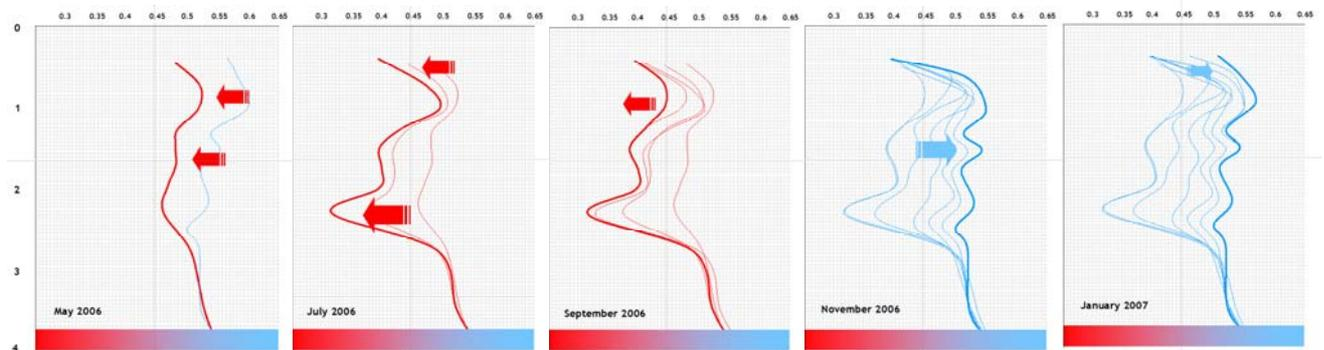
Shallow moisture loss accompanying evaporation can be clearly distinguished from root driven moisture deficit.
