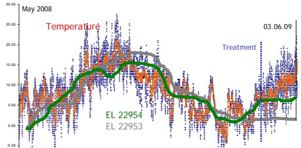
Above is a plot relating temperature to building movement as recorded by the electrolevels and the apparent - yet to be proven - benefit of applying the treatment. Sensor EL 22953 in particular appears to have stabilised.
