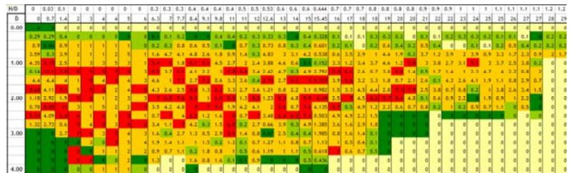
"Looking OK", is fine in such cases. The example we have modelled here is a 16m Oak tree, 9mtrs away from a building on a soil with a Plasticity Index of 45%. The likely stress zone is shaded in red at the bottom of the array.
