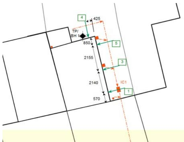
The amplitude of movement also varied. Sensors 4 & 5 rotated by about 0.09 degrees. Sensors 1 & 3, less at around 0.02 degrees but with a variable signature.
