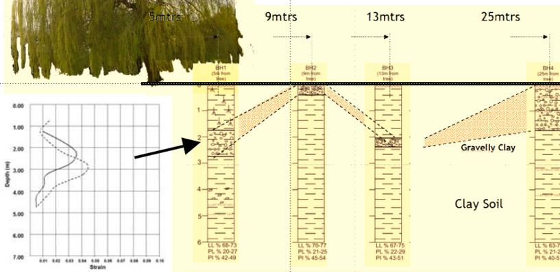
Oedometer, Disturbed –v– Undisturbed. BH 1
