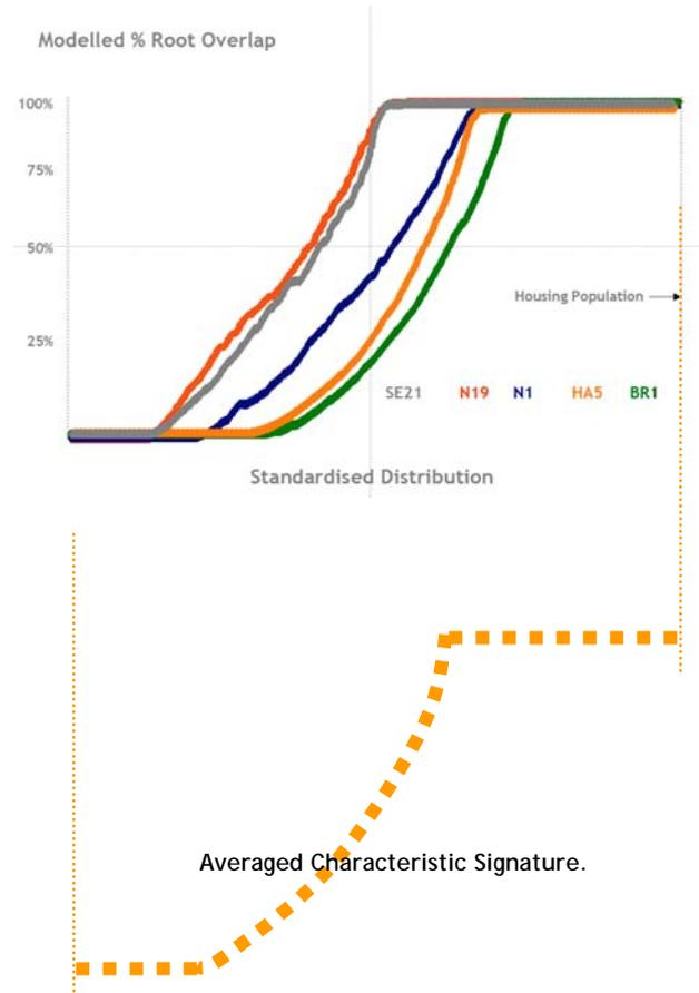
Above is the 'percentage overlap' estimate based on the statistical assessment of root zones encroaching beneath a building derived from claims data.
