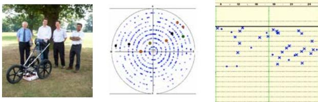
Jon explained that the sensor would only detect roots 5mm in diameter and above. The finer ones - the ones that abstract moisture - can't be detected.
