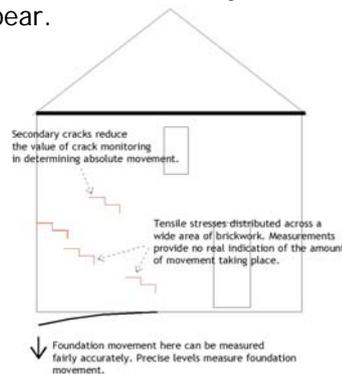
A great deal of research by Burland and Wroth, Skempton and others confirms that masonry panels flex prior to cracking and we have undertaken tests at the MatLab yard to demonstrate this.
