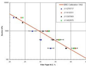
As a result they have identified a batch of filter papers that match the results of the original BRE calibration curve and hope to avoid or reduce the inconsistencies that we sometime see.
