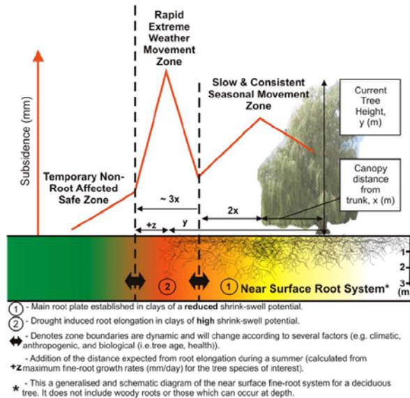
Glenda's work supports the view that the Willow has a dry zone beneath the canopy that produces less movement than at the periphery, where there is enhanced seasonal movement as we see below from precise level survey shown below with an exaggerated 'y' scale.
