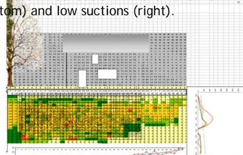
The pattern is consistent with the recent wetter weather and we can model 'what if' scenario in a long, dry summer when the risk would increase. This year we expect 1- 2mm cracks at most.
