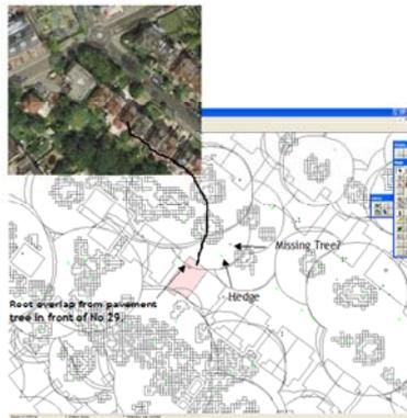
The modelled root zone suggests that the pavement tree is the most likely cause of damage when root zones are plotted.
