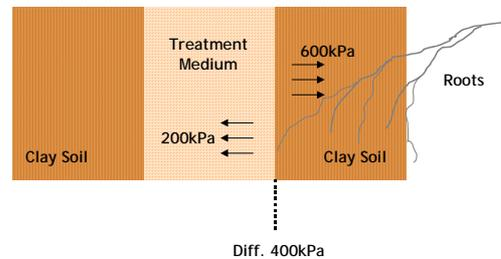
The CRG proposal extends the availability of harvested water and balances suctions in the ground sufficient to induce controlled release, avoiding saturation. In short, it is particularly efficient and designed to deliver moderate water retention properties, allowing water to reach the zone where it is needed to abate or reduce the nuisance.
