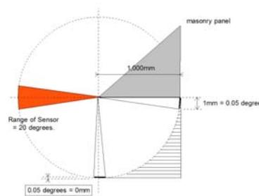
Calibration between vertical and rotational movement is complex as we see, left, but our study suggests that we use a value of 0.2 degrees of rotation as the onset of movement sufficient to cause cracking in a domestic structure.
