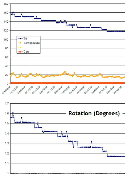
By plotting temperature alongside movement, we can discount it as a cause. Second, because we are measuring fine movement we can detect it much quicker than say, crack or level monitoring.
