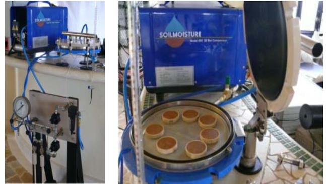
They have undertaken their own calibration using six batches of 12 No. 50mm diameter x 10mm high clay samples placed in the pressure membrane extractor and taken to suctions of 100, 250, 500, 750, 1,000 and 1,500 kPa.
