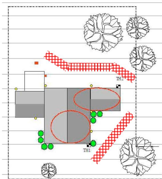
The Oak trees are around 14m high and between 6 - 14mtrs away from the building and matters are complicated by the fact that extensions have been added to three elevations, all with differing foundation depths.
