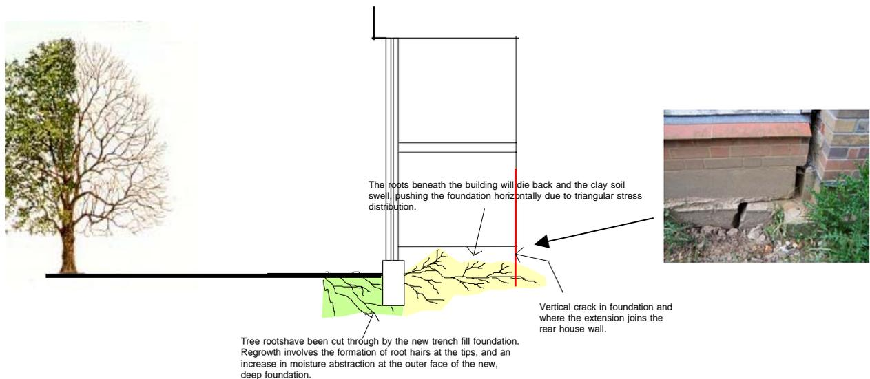
The mechanism is described in a B.R.E. Digest and the correct solution would have been to incorporate compressible boarding on the inner face of the foundation at the time of construction.
