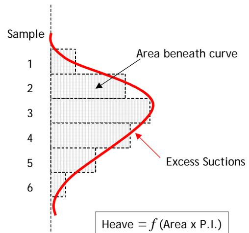
200mm of ground movement would require high suctions over the depth of the bore and soils with a high P.I.
