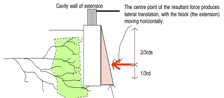
Because of new root growth, the outer face of clay shrinks away seasonally, exhibiting progressive movement as the force from the inner face (beneath the building) prevents closure. Monitoring shows opening in the summer and no movement in the winter.
