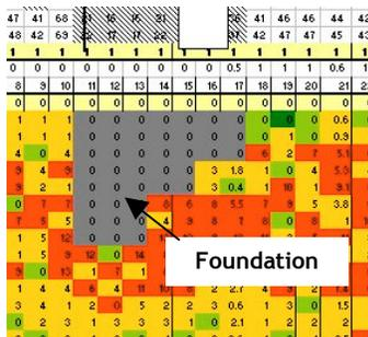
Using the levelling profile (bottom section of above illustrations) we can see how much movement takes place at ground level due to the presence of the tree, and then model 'what if' scenario's. In the middle illustration we have deepened the front house wall (noted by grey cells), and right, underpinned the entire property, reducing the depth as we move away from the tree.
