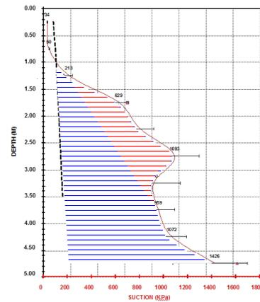
Traditionally, and before adjustment, the laboratory estimate of swell would include the blue shaded area. In fact, the true value is far more likely to be the red area only, and then only if there is support using the moistures to show a deficit coincident with this depth. We better understand the need to adjust the  $K_0$  line to ensure the above doesn't lead to underpinning or tree removal unnecessarily.
