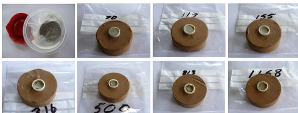
Clive tells us "this technique offers several benefits. The material is easily calibrated in standard oedometers using the void ratio at 100 and 1,000kPa and its properties well published. It is consistent and 1kg of bentonite would do around 2,000 tests. It is more sensitive over the range of suctions we are interested in."
