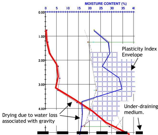
We see the suction profile (red) commences at around 3.25mtrs, and then increases linearly - and quite sharply - until we strike the porous layer represented here by the black broken line. The line isn't characteristic of a root induced problem as it commences a little too deep below ground.
