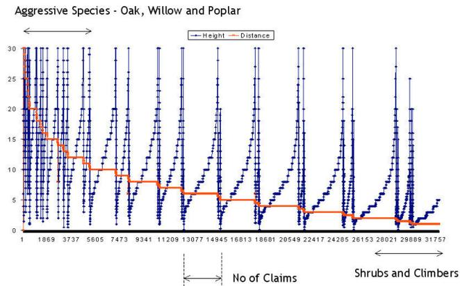
The regular signature across differing height ranges illustrates the point that the average tree poses a threat to a property wherever it is situated within a radius equal to, or less than, the tree height.
