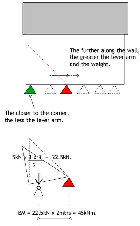
Below we plot the BM (y axis - kNm) at various lengths along the wall (x axis - mtrs). This illustrates one of the modules behind the numeric method of assessing risk using the statistical data from previous pages to utilise the H/D ratios. Plotting the relationship between trees and buildings, knowing the soil type and tree height leads to a scientific method of risk assessment.
