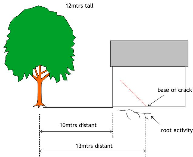
The sketch above illustrates why ‘distance to building’ generally underestimates the influence of the tree. In this case, the tree root influence on the ground (by which we mean the abstraction of moisture from clay soils by roots sufficient to cause damage) is 13mtrs, not 10mtrs. An increase of between 20 - 30% compared with the ‘distance to building’ figure.
