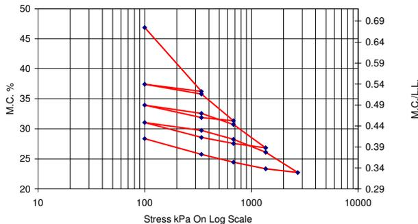
The virgin compression line can be clearly seen with the branching unloading and reloading lines. This is not representative of its undisturbed natural state but it does show the general signature of the consolidation process.
