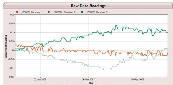
DataREADER suggests an 80% probability that movement reflects root induced clay shrinkage for the 'active sensors' and 45% for the datum. Generally any value less than 70% would be classed as unreliable.
