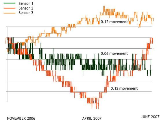
Because we are measuring flexure directly, we have an opportunity of making comparisons with the work of Burland & Wroth and others. It is widely recognised that crack monitoring is of limited use and whilst precise levels measure vertical movement, electrolevels measure how the masonry bends and the amount of flexure needed to exceed the limiting tensile stresses within the wall.
