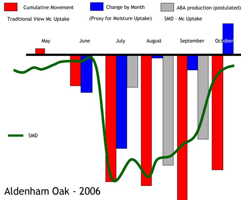
Evaporation forms part of this value, but this is a minor part of the 'moisture loss' equation. The relationship between moisture uptake and ground movement is complex because it isn't linear and varies with the mineralogy of the clay, the health of the tree and climate. We have already examined the water release curve. To simplify matters we can discount the soil mineralogy and health of the tree as the above levels have been taken from one station and share common characteristics.
