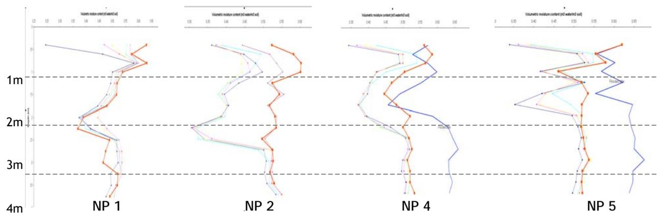
For reference purposes, Station NP 1 is nearest to the tree and NP 5 furthest away. We have omitted the readings from NP 3 due to the variable geology (gravel, sands and clay) and the relatively shallow depth of the bore.
