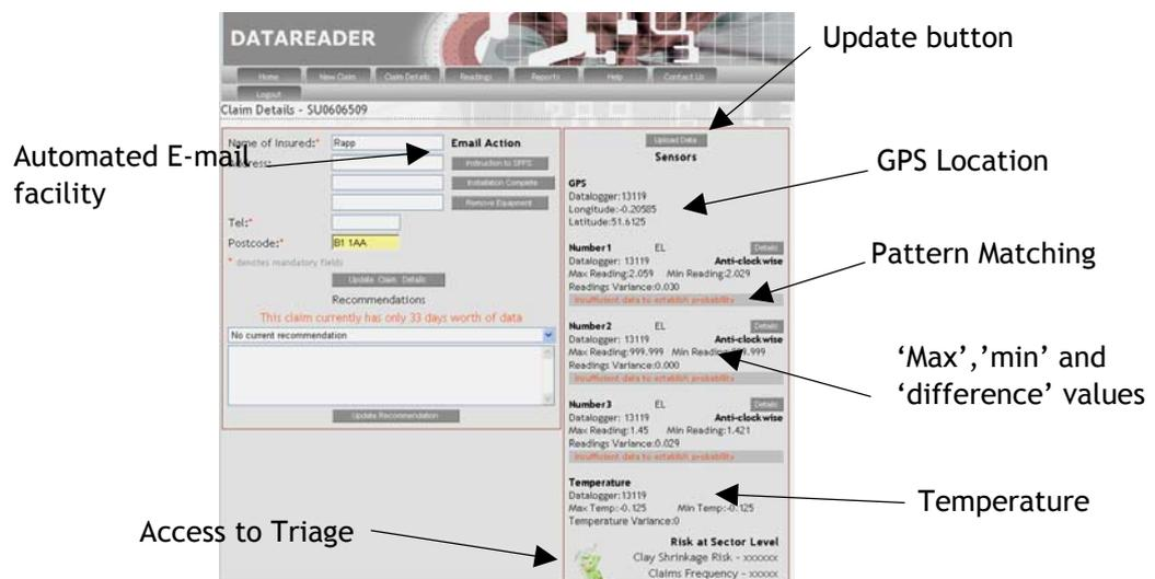
The temperature is also recorded, along with the minimum, maximum and ‘difference’ values. We can see very quickly which parts of the building are moving and which soils are drying more than others.
