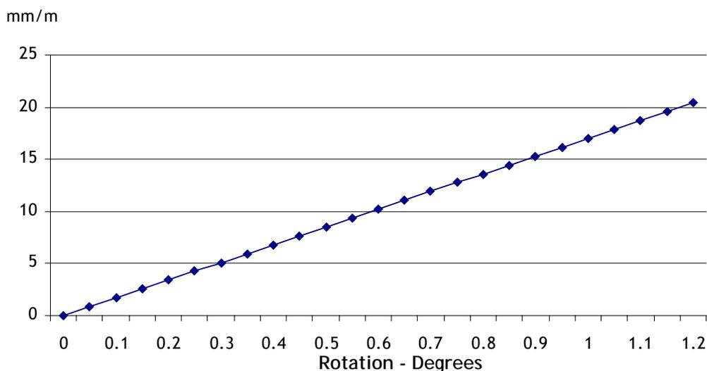
For practical purposes and to exclude minor movements that are encountered on clay soils, but do not result in damage, we suggest a value of 0.01 degrees (that is, 0.17mm of vertical movement over 1m) is regarded as the onset of anything 'significant'. The interpretation would be a difference between the datum and the 'active' station, and should not be regarded as an absolute measure of movement from one sensor alone.
