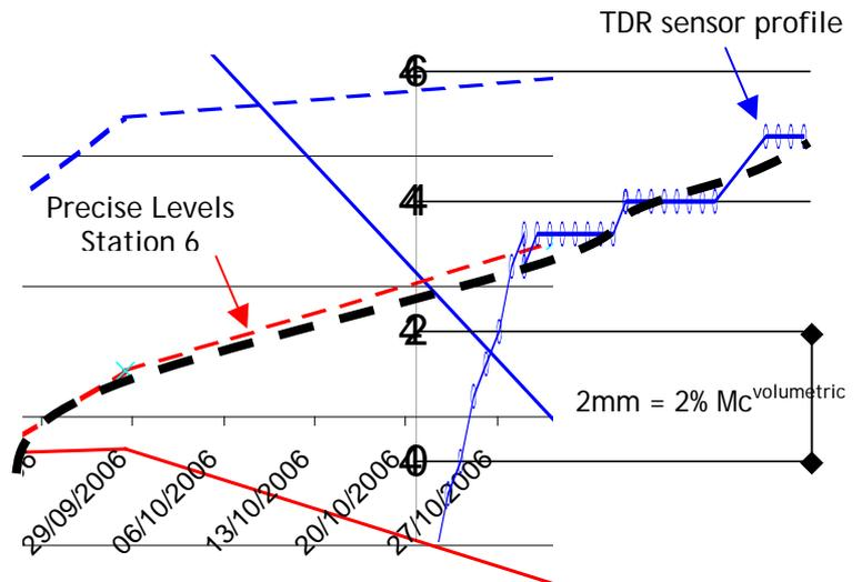
The gradients are very similar (bold broken line) and the project will be looking at correlations to see if we can 'pattern match' over a season. The slope of the line will of course vary with the soil mineralogy and tree species, height and so forth, although we suspect the profile will be fairly constant as suggested by the work of The Building Research Establishment.
