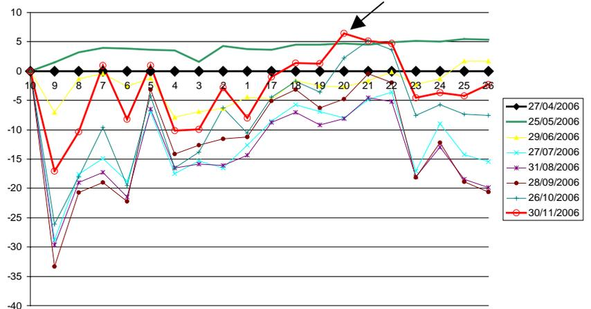
Above we see the results for the end of November. The green line is the high point from May, and the red line is the November reading. We see that at Stations 20 and 21 recovery has already 'lifted' the ground to a point higher than it was in May by nearly 2mm.
