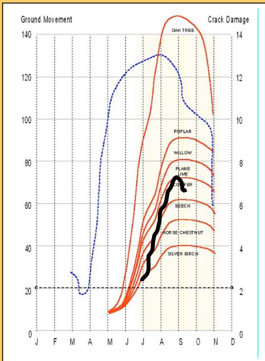
The 'x' axis plots the timescale - January through to December. The vertical axis plots ground movement.
