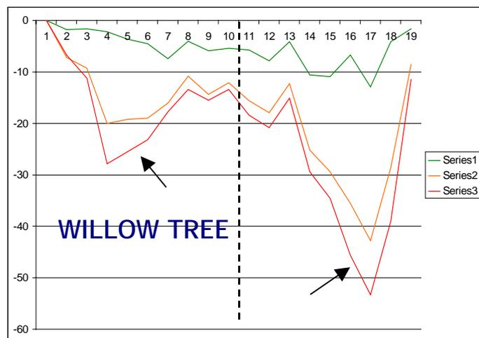
The tree sits in the centre of both graphs (bold dotted line) and the red line (arrowed) plots the latest readings. The results continue to show the presence of a zone of persistent moisture deficiency, and we see less movement directly beneath the tree, but more towards the root periphery as outlined on Page 1.
