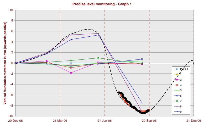
Whereas the levels capture 5 readings over 10 months (one reading every two months on average), electrolevels capture around 100 in 2 months. We can identify the point of contraflexure very quickly, confirming tree root activity as the cause.
