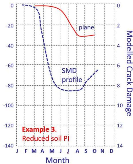
Above, left, a lower SMD reduces the ground movement and damage potential, as does a soil with a reduced plasticity index, above, right. **NB** - the plots are for illustration only – an SMD of 60mm is highly unlikely to deliver ground movement of nearly 30mm
