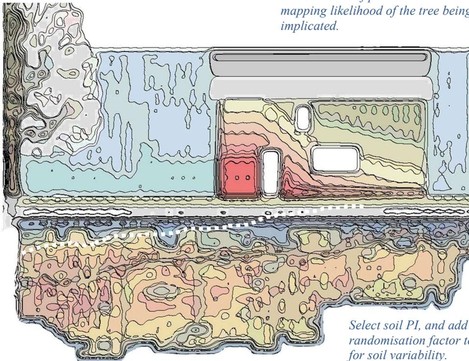
The pattern of soil drying is less structured, reflecting their heterogeneity and accounting for the likely presence of sand lenses, variations in soil PI and root activity with depth. Obviously, this isn’t an accurate map of the exact location of anything. It’s the sum effect at ground level that plots a possible ground movement profile that, if matched with the damage evident, implicates the tree – see white dotted line for ground movement profile.
