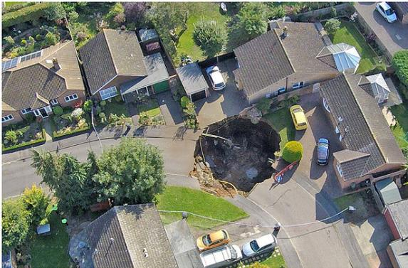
One of the local councillors suggested that the sinkhole could have been caused by a water leak, but the precise cause has yet to be established. Google Street View reveals extensive relaying of the water service beneath the footpath.
