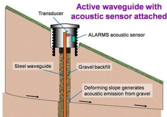
*Image from the web illustrating the method. The waveguide sensor is embedded in gravel. Movement within the gravel emits a noise that is detected by the sensor.*
