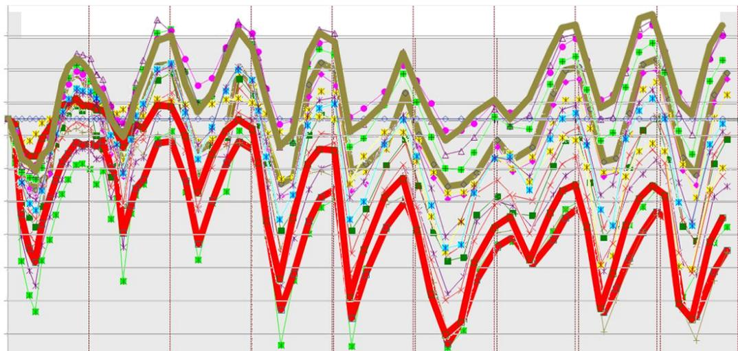
Superimposing array 1 onto array 2 reveals remarkably similar profiles between stations close to the tree and towards the root periphery. Array 1 shows slightly greater recovery closer to the tree (green line) and a greater amplitude of seasonal movement away from it (red line).
