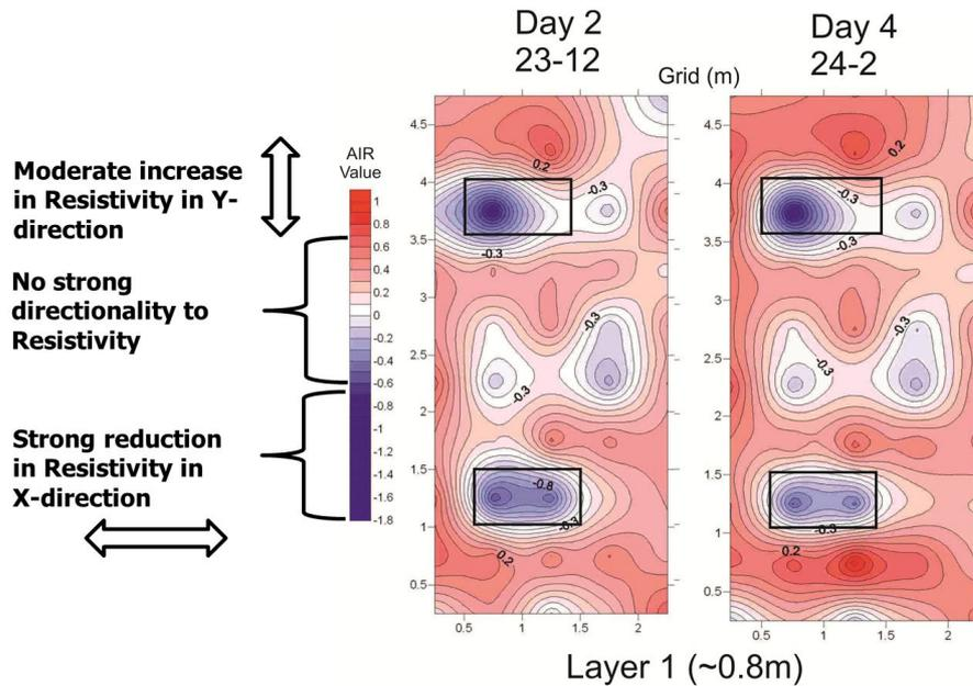
He explains "The above slides show the change in resistivity as a function of its directivity. It shows the "Azimuthal Inhomogeneity Ratio" or "AIR" and is a measure of the x versus y direction dominance in the change in the resistivity value. The side shows that under the plinth the resistivity has dropped and that the 'flow' of fluids causing the drop is predominantly in the X-direction (i.e., matching the electro-kinetic polarisation direction)."
