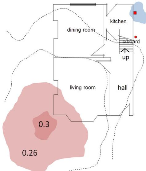
*Tree roots dry soil in the summer, resulting in an increased electrical resistivity*
