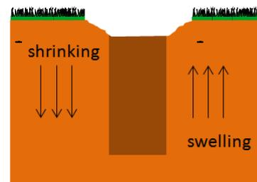
Can the treated zone be 'stable' when surrounded and encased in a shrinking and swelling soil with no slip plane?
