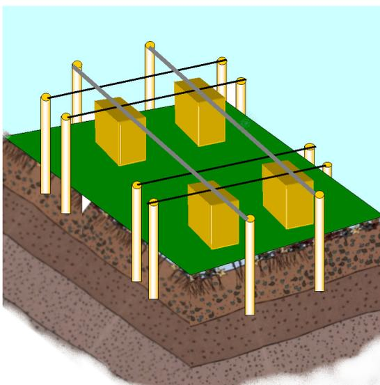
*A diagrammatic of the installation at Aldenham showing the four pad bases. The ground beneath three of the pads was treated and the fourth used as a control.*
