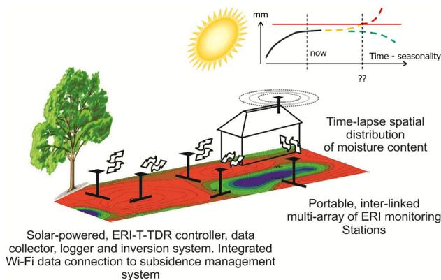
*Monitoring using the Raspberry Pi approach outlined by Nigel. Solar powered arrays gathering data on moisture change in the soil using ER possibly supplemented by electrolevels attached to the face of the building to correlate ground moisture change and building movement over time.*
