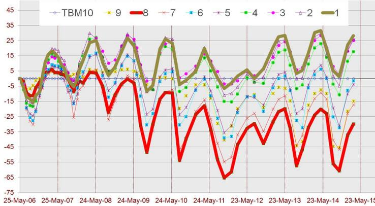
Precise levels taken from the Aldenham willow stations, commencing May 2006. Left, readings along array 1. Station 1 is closest to the tree and station 9 is furthest away. A persistent deficit has developed at the root periphery with some recovery closer to the tree following heavy rainfall in 2012.
