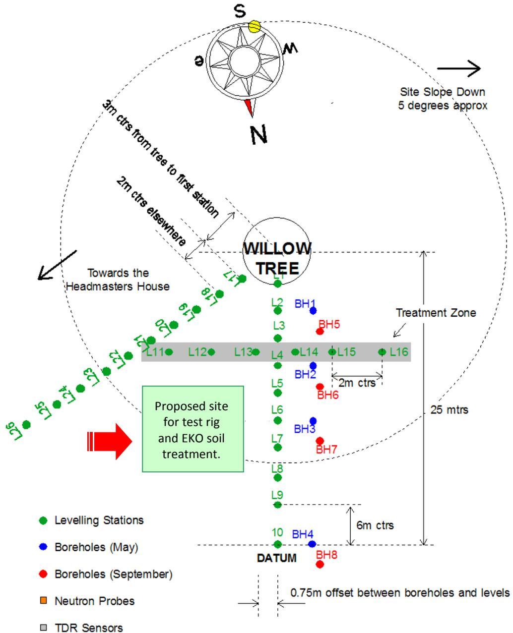
A load frame is to be installed on site at the above location (indicated by a red arrow), between the two levelling arrays. See following pages for details.
