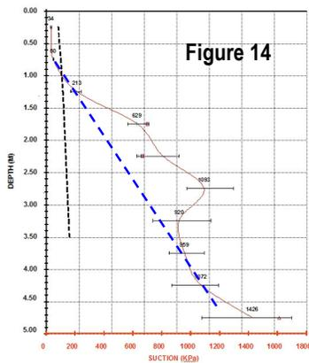
Left we have an example (BH 3, Test\_2, Disturbed) of an anomalous filter paper test result with  $K_0$  plotted as a black dotted line. We would suggest the line should join the upper and lower values – see alternative (blue dotted line).
