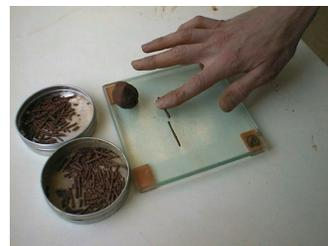
There has been much debate over recent years surrounding the accuracy of testing soils to detect desiccation. Richard Driscoll provided some very useful guidance when he developed a relatively simple test allowing engineers to make an approximate assessment based on comparing the moisture content of the soil with their Plastic and Liquid Limits.
